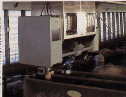
The Feedlogic self-propelled feed delivery unit travels on a rail and dispenses feed automatically.
